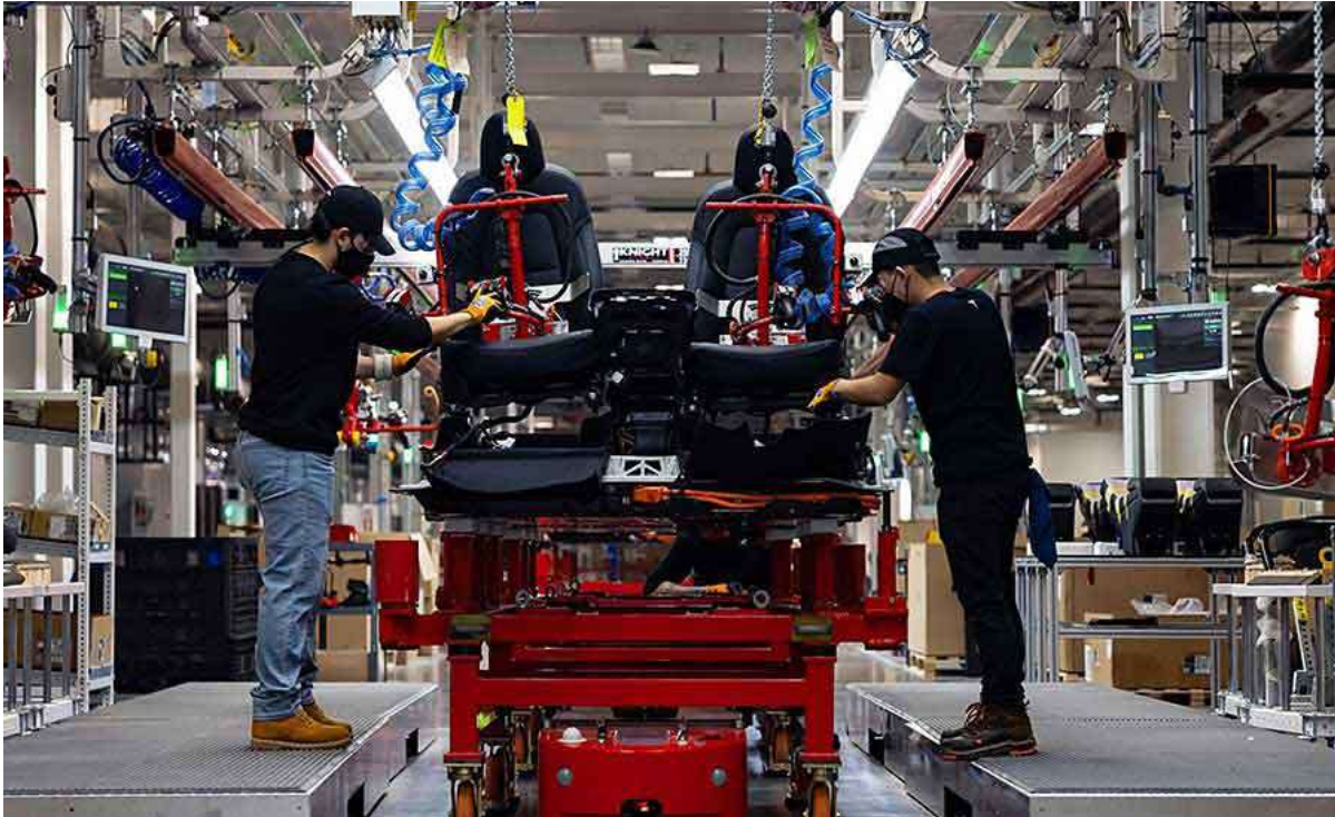
The front seats of the Model Y are attached to the top of a structural battery pack that serves as the floor. Photo courtesy Tesla Inc.
