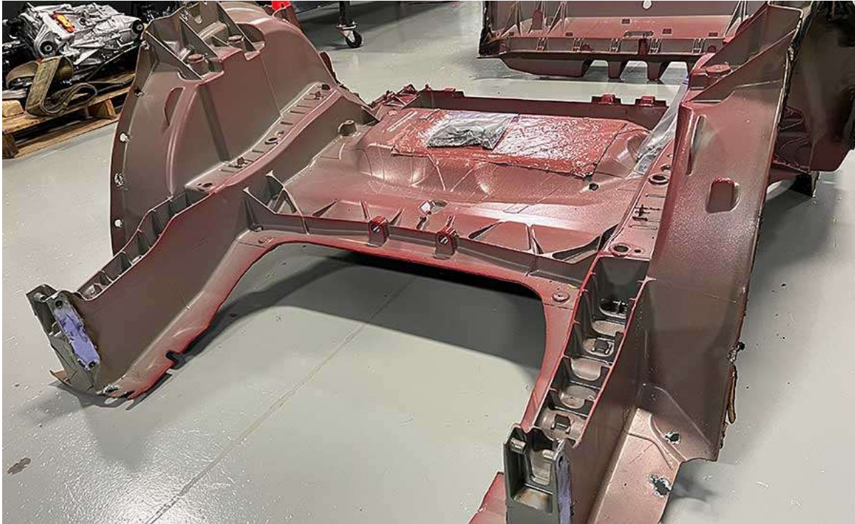
This rear casting used by Tesla simplifies assembly by eliminating hundreds of stamped metal parts. Photo courtesy Munro & Associates
