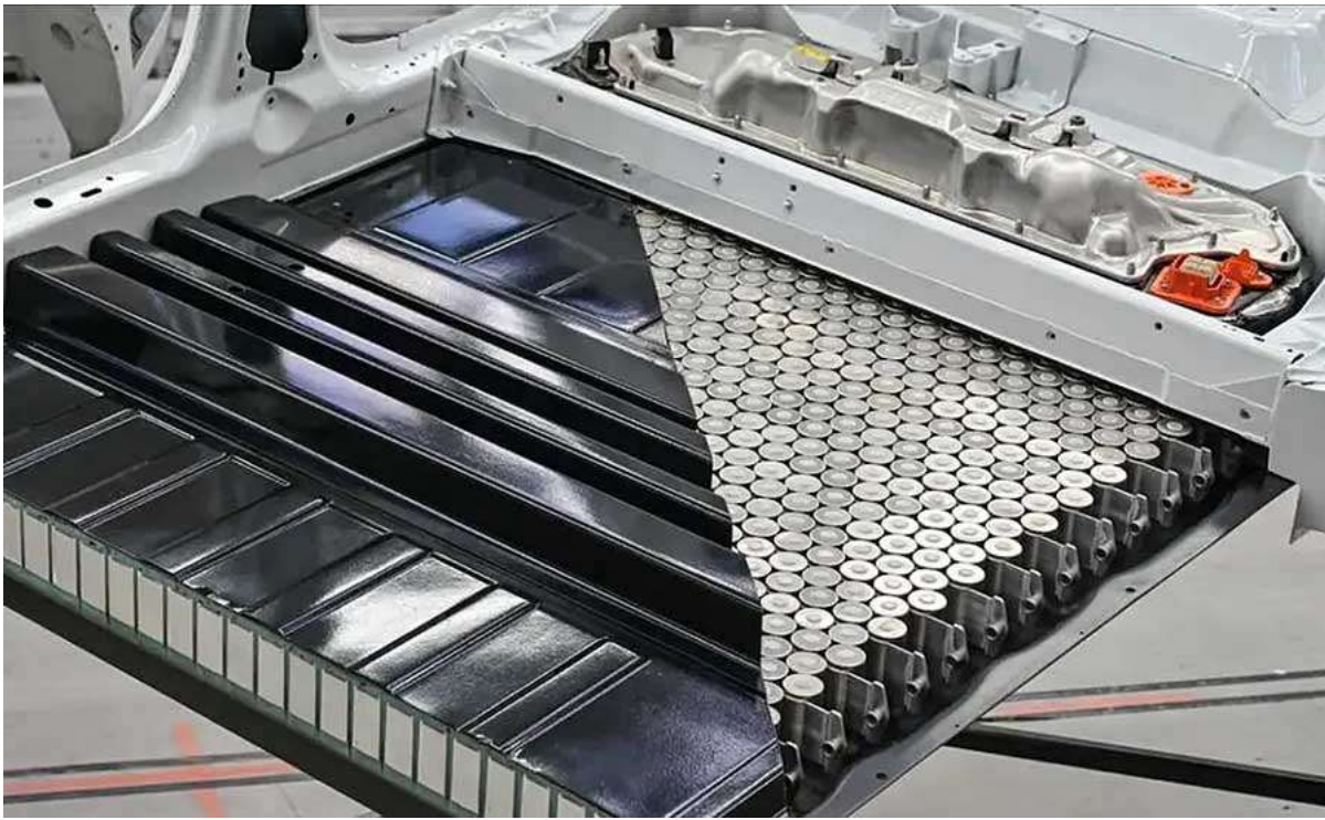
Tesla plans to use more structural batteries that serve as the floor in its vehicles. Illustration courtesy Tesla Inc.
